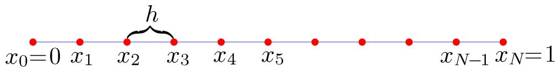
$$S = \{x_i = ih; \quad i = 0, 1, \dots, N\} \quad \dots \text{ síť}; \quad h \dots \text{krok sítě.}$$
