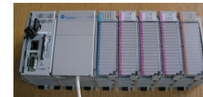
PLC CompactLogix firmy Rockwell
