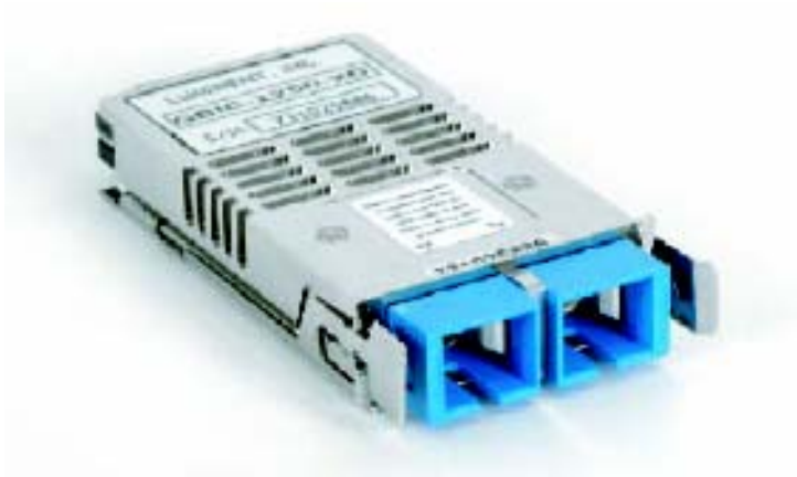
GBIC transceiver (Giga-bit Interface Converter) SC duplex
