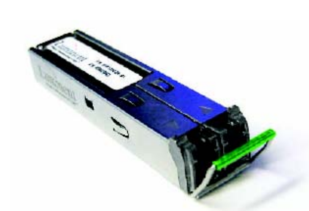
SFP transceiver (Small Formfactor Pluggable) LC duplex (eventuelně MT-RJ)
